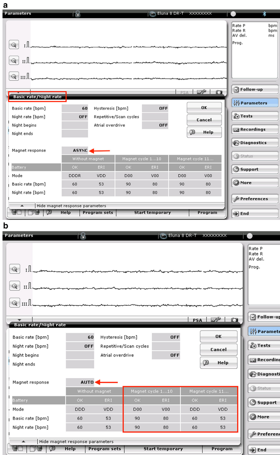
Fig 8. (A) Renamic programmer “parameters” tab from a pacemaker (Eluna 8 DR-T) demonstration patient with the “basic rate/night rate” (red box) selected and the magnet response delineated as “async” (red arrow). (B) Renamic programmer “parameters” tab from a pacemaker (Eluna 8 DR-T) demonstration patient with the “basic rate/night rate” selected. The magnet response—“auto”—is delineated by a red arrow and the “magnet cycles” is highlighted by a red box.
