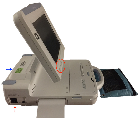
Fig 3. Biotronik Renamic programmer with the power receptacle and on-off switch (red arrow), rear storage compartment (blue arrow), safe programming and emergency shock buttons (red oval), and front storage compartment and untethered stylus (black arrow) highlighted.
